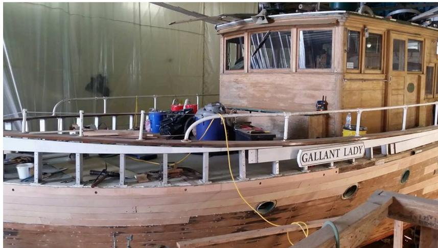
Hull and house wooded, new planks, prepping for paint and varnish.
