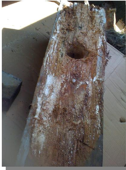
of wood hydrolysis in the horn timber around the rudderpost and keel bolts.
