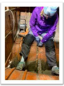
For the bow stem a long section has been removed, scarfs prepared in both ends and we are right now starting on a template to cut a new bow stem. For
