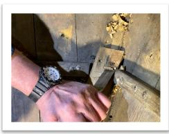
this boat it is best, we have learned, to do the new stem in two pieces that are glued and screwed together, one piece from the inside that is sitting on the
