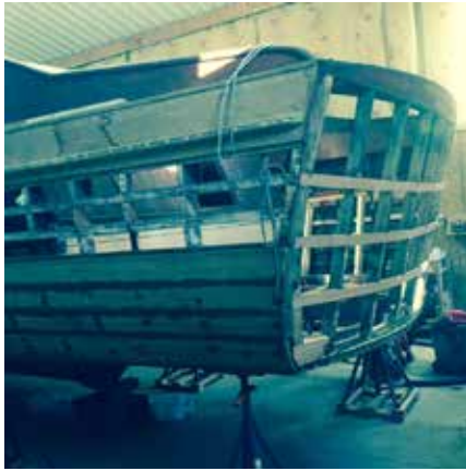
The aft stern and transom of #40626 before replacing ribs and planks.
